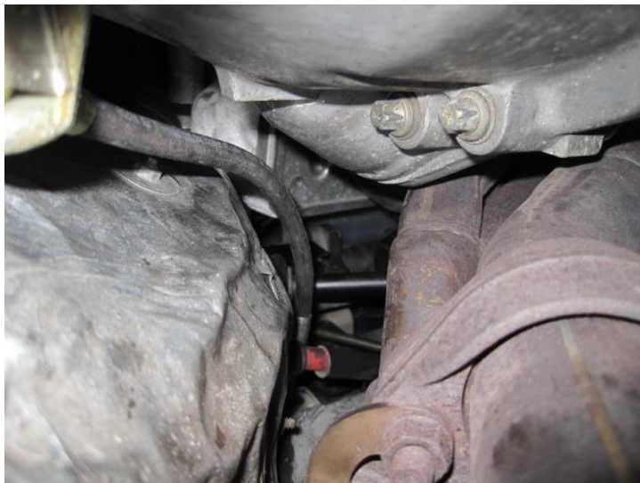
The hydraulic hose goes up between the firewall and the ALPINA header.
