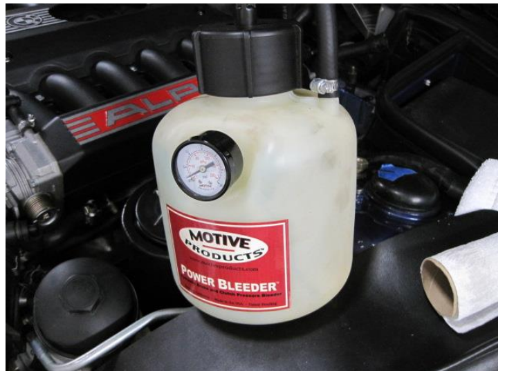
The Clutch Master Cylinder, Hydraulic Hose and Clutch Slave were bled using a Power Bleeder.
