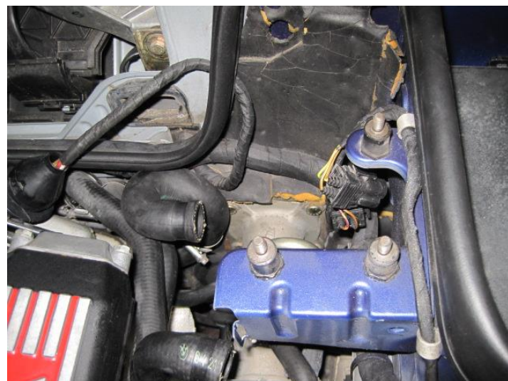
Did I say it was down there... somewhere? A better view with the Aux Water Pump and Positive Jump Terminal removed.
