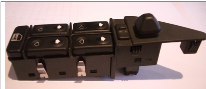
Figure 1: Window Combination switch unit from E31
