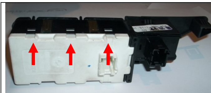
Figure 2: Window Combination switch block (underside view)
