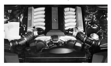
In 1993, BMW realized that 300 horses in something weighing 1790kg wasn't going to cut it with the Wolf of Wall Street crowd. So they ramped up the capacity of that V12 from 5.0 liters to 5.6 liters, tweaked to produce 381bhp and 406lb ft. Meet the 850 CSI, which was only available with a manual gearbox. That new-found power was enough to cut the 0-62mph sprint down from 6.8 seconds to under six seconds. Much more like it.
