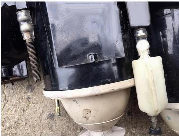
What you have done is to replace the hard plastic parts that are known to brake and fail with plastic tubing that is flexible and very long lasting. It takes a lot of force to pull the tubing off so it is not likely they will ever fail. The tubing also insulates the headlight from vibration and is a simple proven solution used by BOSCH and HELLA for many years and a simple and very inexpensive cure to an extremely common and expensive E31 headlight problem.
