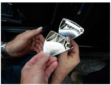
E31 seat flipper - redesigned (on top) vs broken unit
