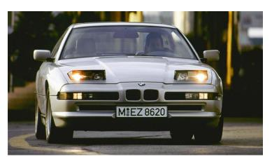
In 1994, BMW shuffled its 8-Series cards; with the range-topping 850 CSI coming on tap, the old 850 was dropped, its place filled with a new 850 CI with a 5.4-litre V12, 326bhp and a new five-speed auto.
