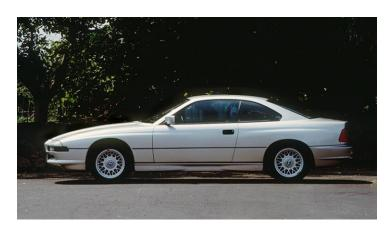
That's the middle pillar at the end of the front side windows, and BMW designed the 8-Series without it, allowing a clean sweep of glass from front to back. Cleaner, cooler.
