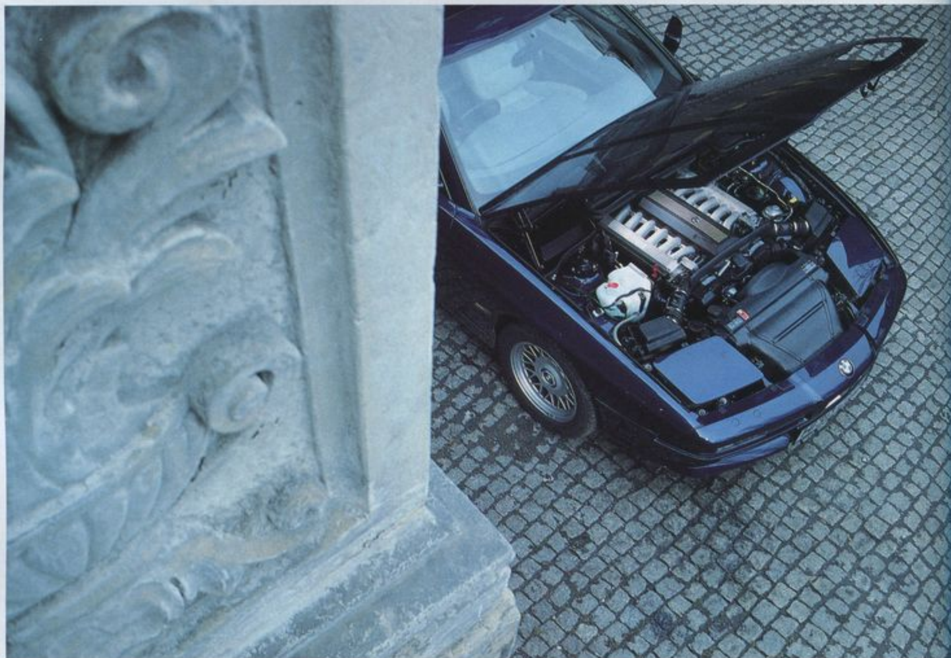
BMW's 5.0-litre V12 engine gives 300bhp at 5200rpm, and 325lb ft of torque at 4100rpm. Flooring the throttle always gives turbine-like acceleration
