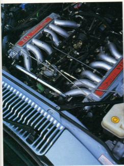
Jaguar V12 is stroked to 6.0 litres; gives smooth 350bhp and thunderous performance. XJR-S chassis and steering are substantially tauter than standard XJS. Cockpit is hedonistic though hardly efficient
