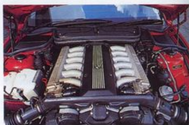
The 5-litre V12 has low friction bores, a seven bearing crank and Bosch Motronic injection and ignition
