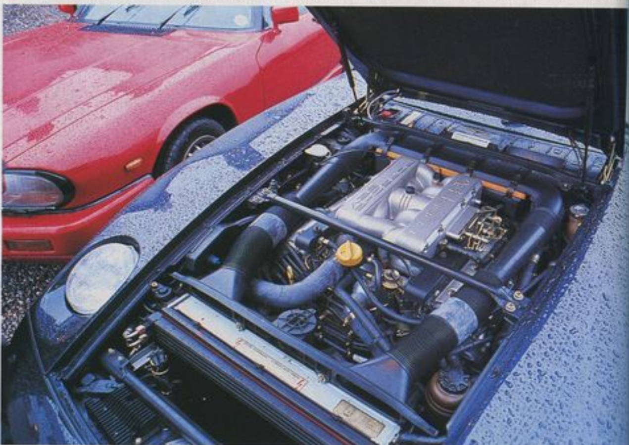
● Heart of latest Porsche 928 is magnificent 32-valve 5-litre V8, good for 320bhp
