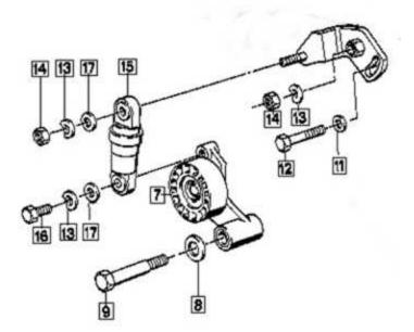
I tem 7 is probably what's causing the screech - a worn tensioner pulley bearing. I'd recommend replacing both this and the tensioner piston, item 15, at the same time.
