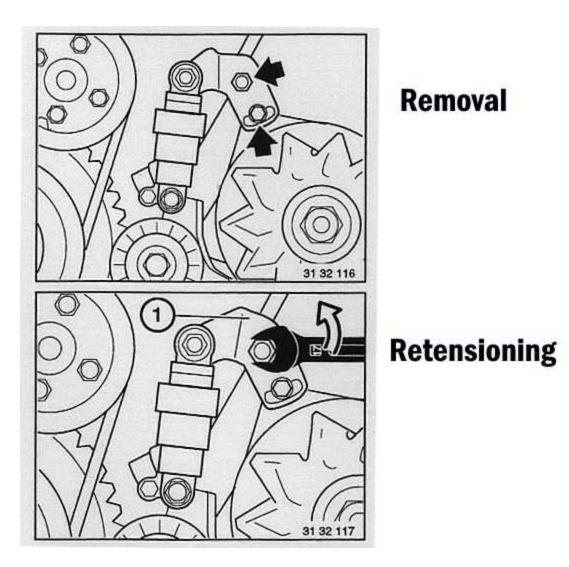
Once released, you can remove these two nuts and a single bolt below and the entire assembly will come free. Replacement is the same, but you need to re-tension the belt by placing an open end on the larger of the two top nuts and turning to the left. At the same time, tighten the lower lock nut. Here's another picture:
